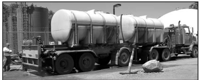
*An RCOC brine tanker fills up at one of the three RCOC brine wells prior to doing dust control.*
