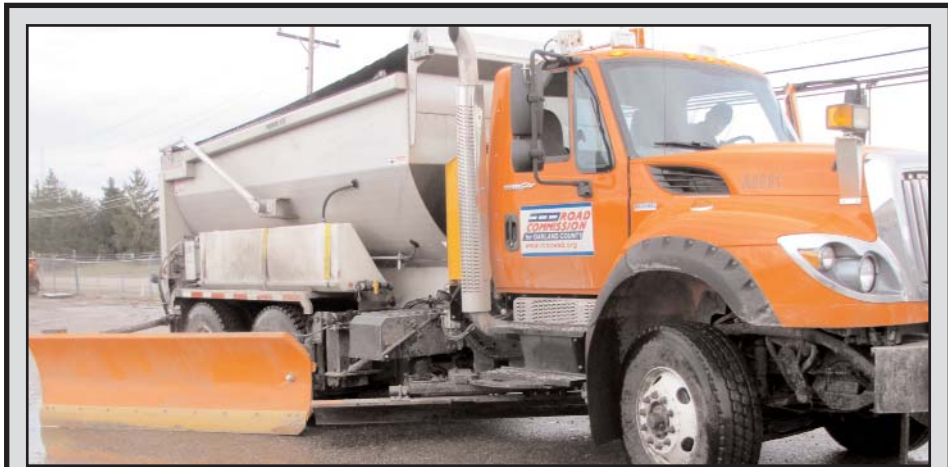
An RCOC plow truck equipped with the new wing plow.
